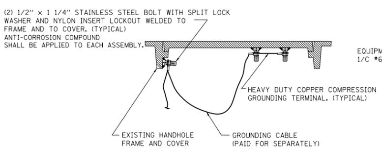
**EXISTING HANDHOLE COVER & FRAME - GROUNDING DETAIL**
