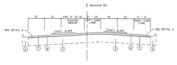
PROPOSED TYPICAL SECTION MEACHAM RD. STA. 57+28 TO 64+09 (NORTH LEG. FACING SOUTH AND INTERSECTION)
