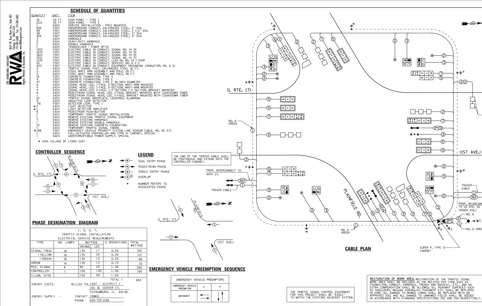
CABLE PLAN, SCHEDULE OF QUANTITIES, PHASE DESIGNATION DIAGRAM & EVP SEQUENCE IL ROUTE 171 (1ST AVE.) AT PLAINFIELD ROAD SCALE: N.T.S. SHEET NO. OF SHEETS STA.
