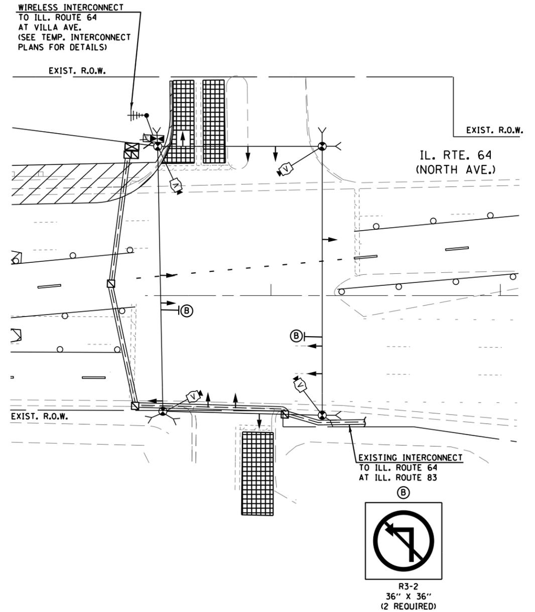
**SIGNAL HEAD PLACEMENT FOR STAGE 2**
