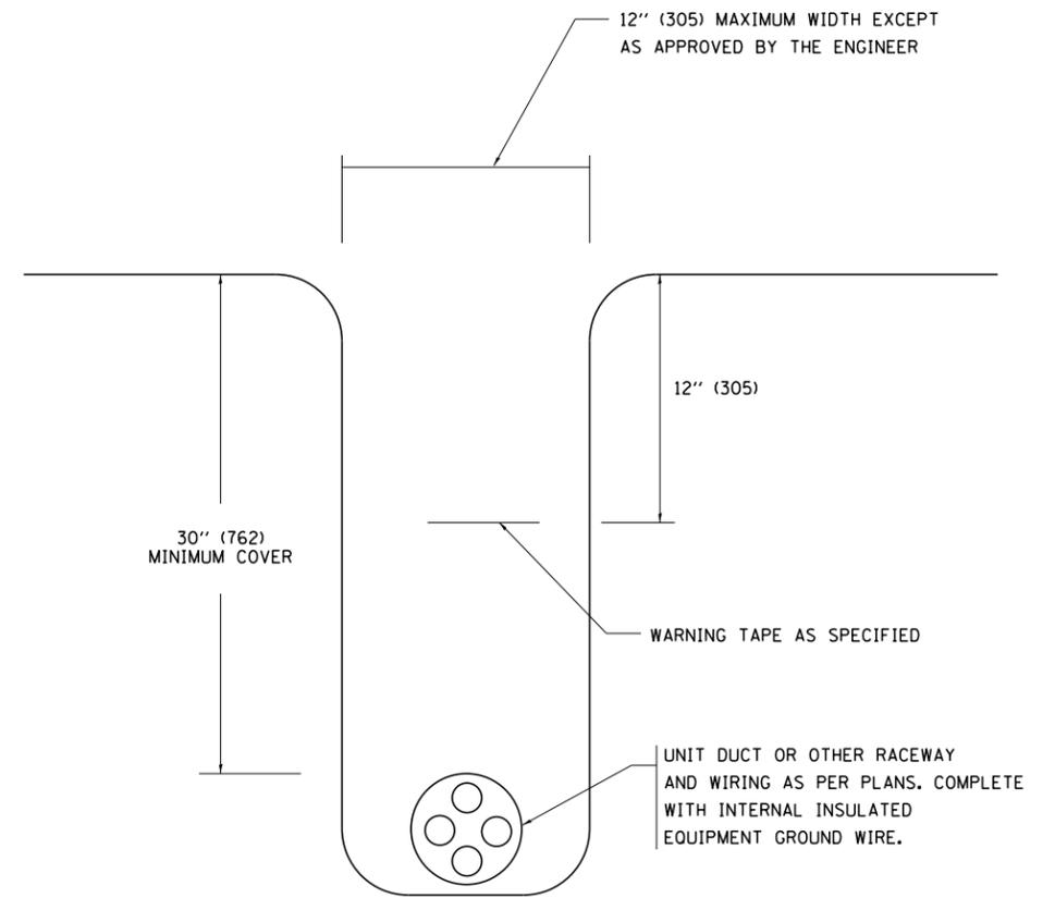
**TYPICAL WIRING IN TRENCH DETAIL**
