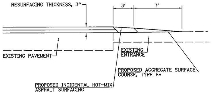
\*AGGREGATE SURFACE COURSE WILL BE INSTALLED FOR EARTH ENTRANCES AT THE ENGINEER'S DISCRETION
