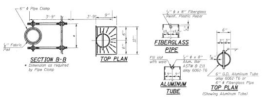
The exterior surfaces of the floor drains shall be painted with the finish coat as specified in the special provisions for Cleaning and Painting New Metal Structures. The exterior surfaces of the drains shall be cleaned according to Steel Structures Painting Council's Spec. SSPC-SP1 prior to painting. Fiberglass pipe shall conform to ASTM D 2996, with short-time rupture strength hoop tensile stress of 30,000 p.s.i. minimum.
