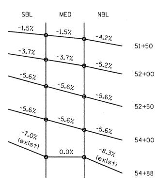
SBL and MED Transition from -1.5% AT 51+50 to -5.6% at 52+50 -5.6% at 54+00 to matching existing at 54+50.
