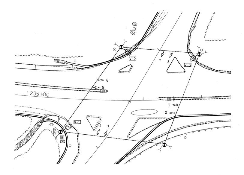
THE CONTRACTOR SHALL COORDINATE THE PLACEMENT OF WOOD POLES, GUY WIRES, AND OTHER TEMPORARY TRAFFIC SIGNAL EQUIPMENT WITH THE ENGINEER TO PREVENT CONFLICTS WITH CONSTRUCTION STAGING AND OVERHEAD UTILITIES.
