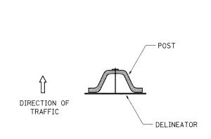
DELINEATORS SHALL BE INSTALLED ACCORDING TO STANDARD 635001 EXCEPT THAT THE POST SHALL BE ROTATED 180°. THE POST WILL HAVE THE WIDE SIDE FACING TRAFFIC AND THE DELINEATOR ATTACHECD AS SHOWN ABOVE.
