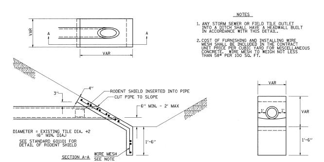
SLOPE WALL FOR FIELD TILE OUTLETS
