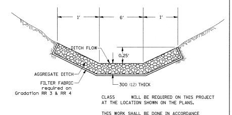
WITH SECTION 283. AGGREGATE DITCH WILL BE MEASURED FOR PAYMENT IN PLACE AND THE AREA COMPUTED IN SQUARE METERS (SQUARE YARD) OF ACTUAL SURFACE AREA. AGGREGATE DITCH WILL BE PAID FOR AT THE CONTRACT UNIT PRICE PER SQUARE METER (SQUARE YARD) FOR AGGREGATE DITCH. 300 mm(12").
