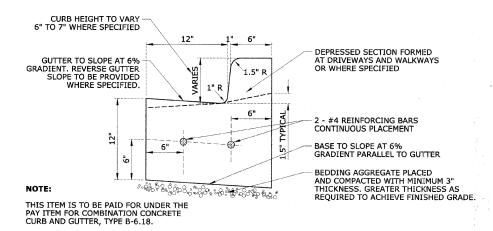
4" TO 8" WHERE SPECIFIED, GUTTER TO SLOPE AT 6% GRADIENT; REVERSE GUTTER SLOPE TO BE PROVIDED DEPRESSED SECTION FORMED AT DRIVEWAYS AND WALKWAYS OR WHERE SPECIFIED 2 - #4 REINFORCING BARS, CONTINUOUS PLACEMENT BASE TO SLOPE AT 6% GRADIENT - BEDDING AGGREGATE PLACED AND COMPACTED WITH MINIMUM 3" THICKNESS; GREATER THICKNESS AS REQUIRED TO ACHIEVE FINISHED GRADE
