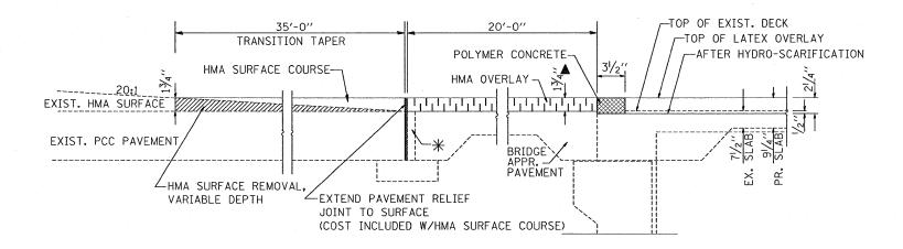
APPROACH PAVEMENT OVERLAY CROSS SECTION
