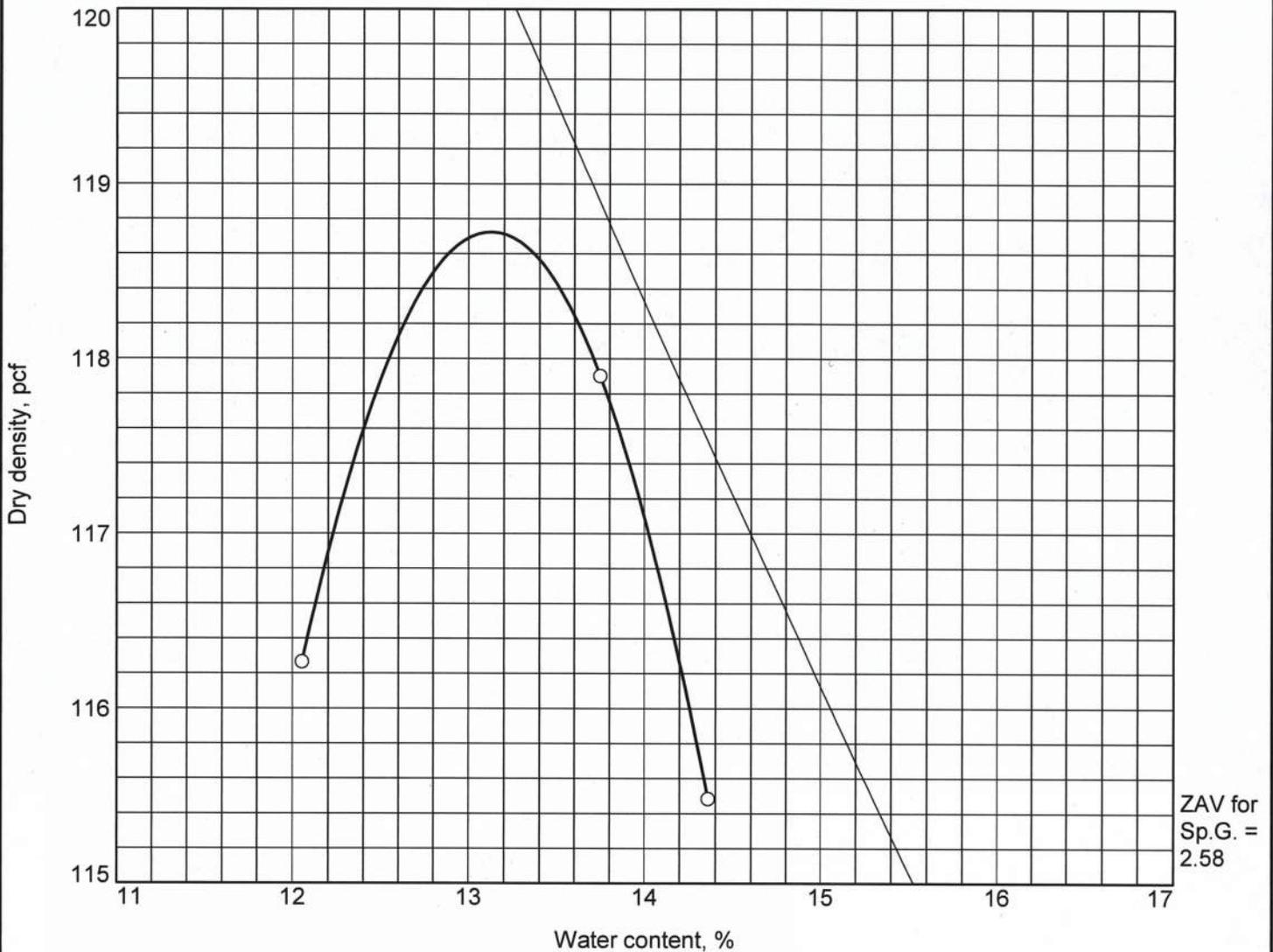
Test specification: ASTM D 698-12 Method B Standard
