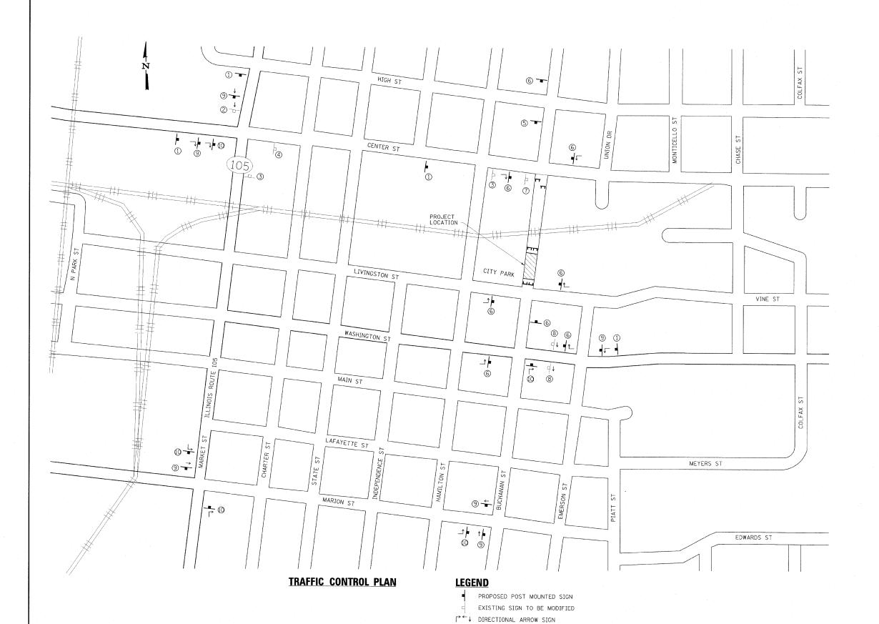
1,2,ETC. SIGN NUMBER SEE DETAILS ROAD CLOSED TO ALL TRAFFIC TT ROAD CLOSED TO THRU TRAFFIC
