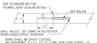
BARS SHALL BE EPOXY COATED; #6 DEFORMED, 24" LG. AT 24" CTRS. FOR LONG CONST. JT. #6 DEFORMED, 24" LG. AT 18" CTRS. FOR TRANS. CONST. JT. CONSTRUCTION JOINT
