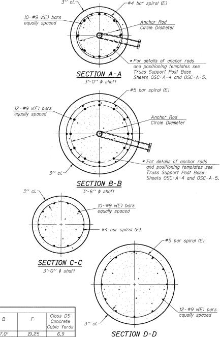
The foundation dimensions shown in the Foundation Design Table are based on the presence of mostly cohesive soils with an average Unconfined Compressive Strength (Qu) of at least 1.25 tsf, which must be determined by previous soil investigations at the jobsite. When other conditions are indicated, the boring data will be included in the plans and the foundation dimensions shown in the Foundation Data Table will be the result of site specific designs.
