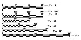
ENGINEERING SCALES. REDUCED SIZED PLANS WILL NOT CONFORM TO STANDARD SCALES. IN MAKING MEASUREMENTS ON REDUCED PLANS, THE ABOVE SCALES MAY BE USED.
