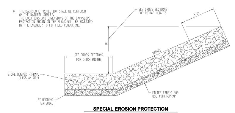
LIMITS OF THE RIPRAP ARE DETERMINED IN THE FIELD BY THE ENGINEER.
