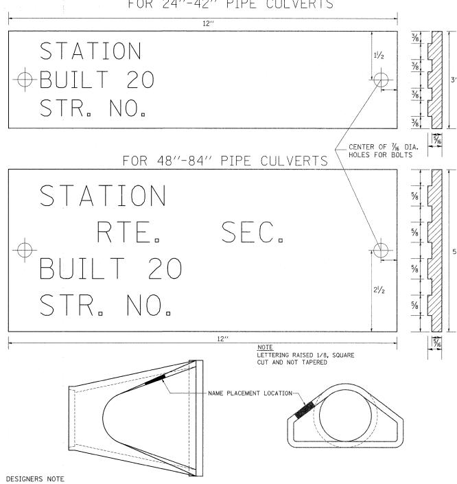
NAME PLATES SHALL BE FURNISHED & INSTALLED ACCORDING TO SECTION 515 OF THE STANDARD SPECIFICATIONS, EXCEPT 2 BOLTS SHALL BE USED TO FASTEN THE PLATE TO THE END SECTION.
