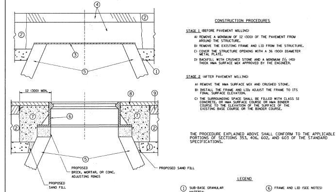
EXISTING BROKEN FRAMES AND LIDS SHALL BE REMOVED AND DISPOSED OF BY THE CONTRACTOR AND SHALL BE REPLACED AS DIRECTED BY THE ENGINEER. REPLACEMENT FRAMES AND LIDS WILL BE PAID FOR IN ACCORDANCE WITH ARTICLE 109,04 OF THE STANDARD SPECIFICATIONS UNLESS A SEPARATE PAY ITEM HAS BEEN PROVIDED.
