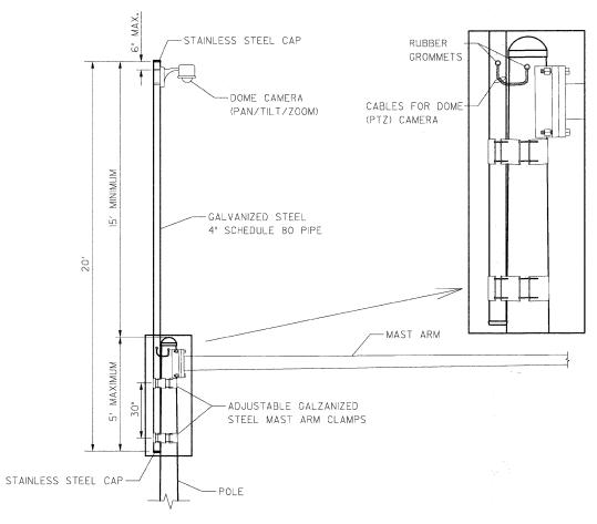
CAMERA MOUNTING ASSEMBLY DETAIL
