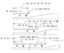
\* TURN LANES IN EXCESS OF 400' (120 m) IN LENGTH MAY HAVE AN ADDITIONAL SET OF ARROW - "ONLY" INSTALLED MIDWAY BETWEEN THE CHER TWO SETS OF ARROW - "ONLY".
