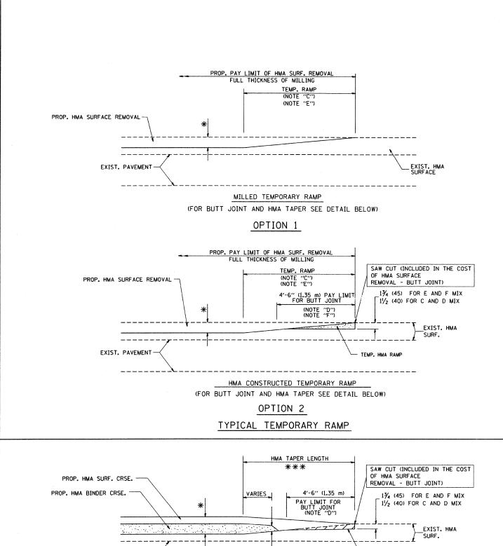
HMA SURF, REMOVAL - BUTT JOINT BUTT JOINT AND HMA TAPER TYPICAL BUTT JOINT AND HMA TAPER FOR MILLING AND RESURFACING
