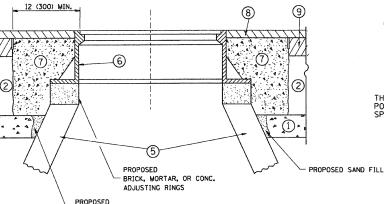
EXISTING BROKEN FRAMES AND LIDS SHALL BE REMOVED AND DISPOSED OF BY THE CONTRACTOR AND SHALL BE REPLACED AS DIRECTED BY THE ENGINEER. REPLACEMENT FRAMES AND LIDS WILL BE PAID FOR IN ACCORDANCE WITH ARTICLE 109.04 OF THE STANDARD SPECIFICATIONS UNLESS A SEPARATE PAY ITEM HAS BEEN PROVIDED.
