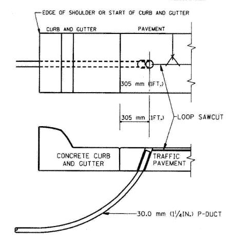
CURB AND GUTTER LOOP LEAD-IN TRANSITION DETAIL
