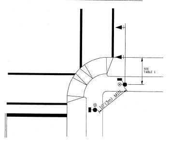
RECOMMENDED PUSHBUTTON LOCATIONS FOR ACCESSIBLE PEDESTRIAN SIGNALS SHALL BE IN ACCORDANCE WITH THE CURRENT MUTCO (SEE NOTE 1). TO MEET MUTCD REQUIREMENTS, PEDESTRIAN SIGNAL PUSHBUTTONS MAY HAVE TO BE MOUNTED ON A SEPARATE POST.
