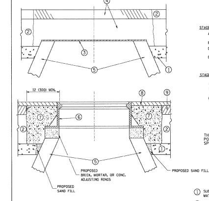
EXISTING BROKEN FRAMES AND LIDS SHALL BE REMOVED AND DISPOSED OF BY THE CONTRACTOR AND SHALL BE REPLACED AS DIRECTED BY THE REGINEER. REPLACEMENT FRAMES AND LIDS WILL BE PAID FOR IN ACCORDANCE WITH ARTICLE 109.04 OF THE STANDARD SPECIFICATIONS UNLESS A SEPARATE PAY ITEM HAS BEEN PROVIDED.
