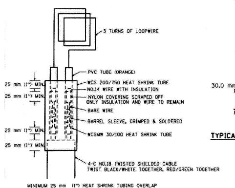
ON WIRE, PVC & SHIELDED CABLE TO FORM WATER TIGHT SEAL
