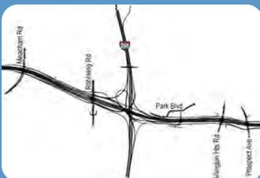
Four-level system interchange with westbound to southbound loop ramp and direct access to Park Boulevard from north, south, and west
