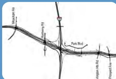
Four-level system interchange and direct access to Park Boulevard from north, south, and west and from Park Boulevard to the north, south (loop ramp), and west via frontage road
