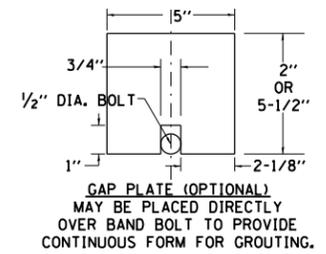
GAP PLATE (OPTIONAL) MAY BE PLACED DIRECTLY OVER BAND BOLT TO PROVIDE CONTINUOUS FORM FOR GROUTING.
