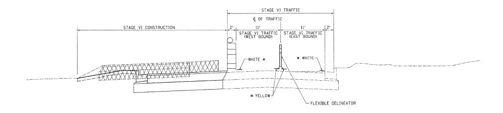
\* ALL PAVEMENT MARKING TAPE IS TYPE III WITH COLOR OF TAPE SHOWN ON TYPICALS SEE SCHEDULE FOR PAINT PAVEMENT MARKING LOCATIONS
