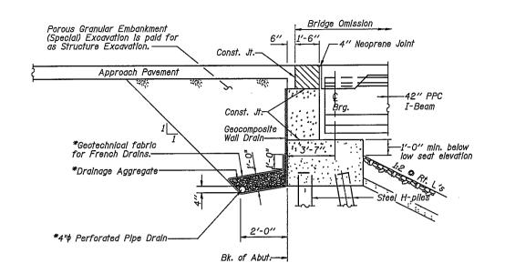
\*Included in the cost of Pipe Underdrains for Structures.
