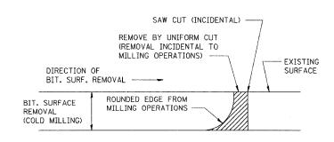
NOTE: WHEN MILLING OPERATIONS PRODUCE A ROUNDED EDGE, THEN A SAW CUT SHALL BE USED TO MANUFACTURE A PERPENDICULAR EDGE AS SHOWN IN THE DETAIL. THE ENGINEER SHALL BE THE SOLE JUDGE CONCERNING THE USE OF THIS DETAIL
