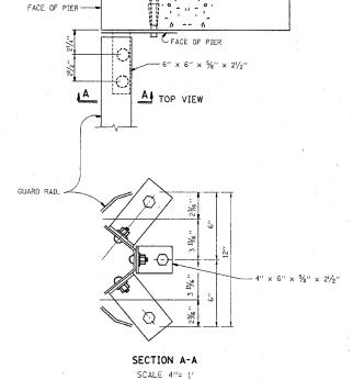
DETAIL OF CONNECTION OF GUARDRAIL TO SQUARE BRIDGE PIER OR FOUNDATION.
