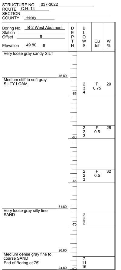
SPT. (N) = Sum of last two blow values in sample. (Qu) B=Bulge S=Shear P=Penetration Test Stations, Depths, Offset, and Elevations are in Feet
