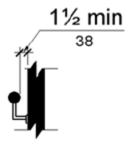
Gripping Surface. Handrail gripping surfaces shall be continuous along their length and shall not be obstructed along their tops or sides. The bottoms of handrail gripping surfaces shall not be obstructed for more than 20 percent of their length. Where provided, horizontal projections shall occur 1½ (38 mm) minimum below the bottom of the handrail gripping surface.
