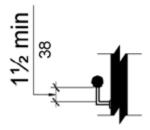
Circular Cross Section. Handrail gripping surfaces with a circular cross section shall have an outside diameter of 1½ inches minimum and 2 inches maximum.
