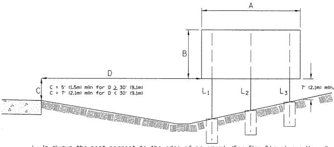
L<sub>1</sub> Is always the post nearest to the edge of pavement. (See Sign Structures Manual)
