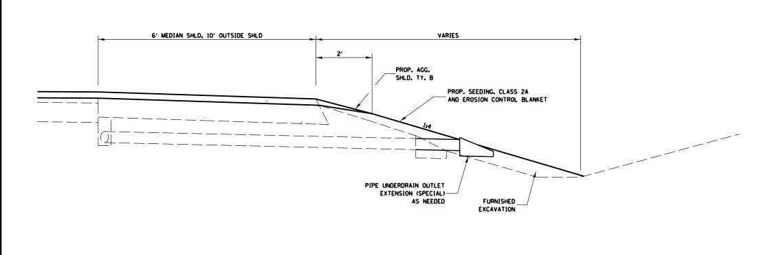
USER NAME = \$USER\$ DESIGNED -REVISED -PIPE UNDERDRAIN STATE OF ILLINOIS REVISED \$FILEL\$ DRAWN OUTLET EXTENSION (SPECIAL) DETAIL PLOT SCALE = \$SCALE\$ CHECKED -**DEPARTMENT OF TRANSPORTATION** REVISED -PLOT DATE = \$DATE\$ DATE REVISED -SCALE: SHEET OF \_\_\_ SHEETS STA.\_
