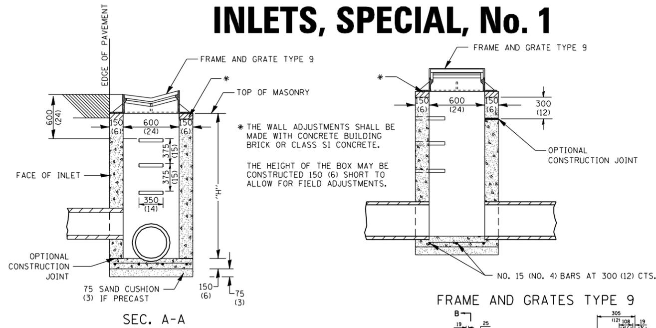
\* THE WALL ADJUSTMENTS SHALL BE MADE WITH CONCRETE BUILDING BRICK OR CLASS SI CONCRETE.
