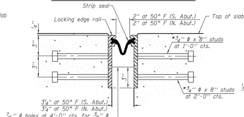
SECTION THRU WELDED RAIL JOINT AT ROADWAY
