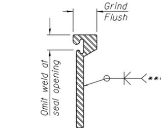
\*\*\* Back gauge not required if complete joint penetration is verified by mock-up.
