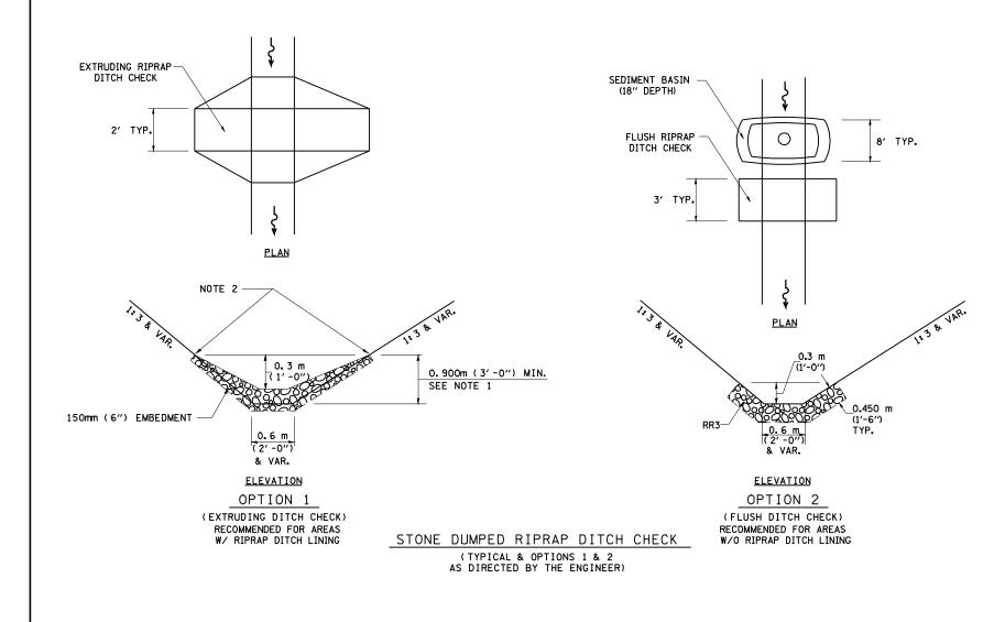
NOTE 1: RIPRAP SHALL EXTEND FAR ENOUGH UP THE SLOPES TO ALLOW O.3m (1') OVERTOPPING TO AVOID ERODING AROUND THE EDGES OF THE RIPRAP
