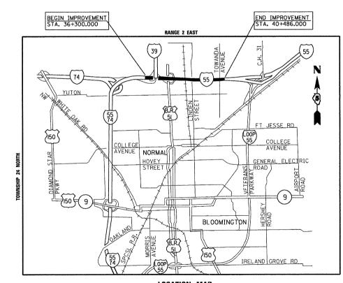
STRUCTURE DESCRIPTION (57-4)HBR-3 STRUCTURE NO. 057-0235 (N.B.) & 057-0236 (S.B.). BRIDGE LENGTH 46.168 m. THREE SPAN CARRYING F.A.I. 55 OVER LINDEN STREET & STATION 38+544.044. BRIDGE STRUCTURE TO BE REMOVED & REPLACED.
