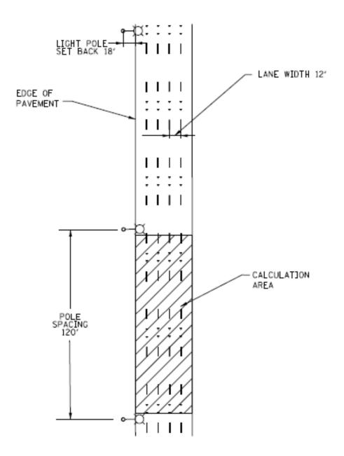
The selected luminaire shall meet the following Luminaire Performance Table:
