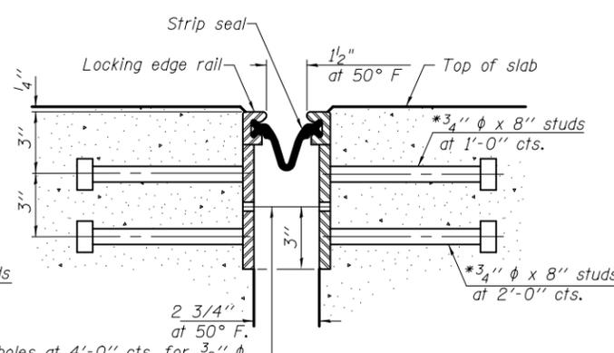
7/16"  $\phi$  holes at 4'-0" cts. for 3/8"  $\phi$  bolts. All bolts shall be burned, sawed, or chipped off flush with the plates after forms are removed, typ.
