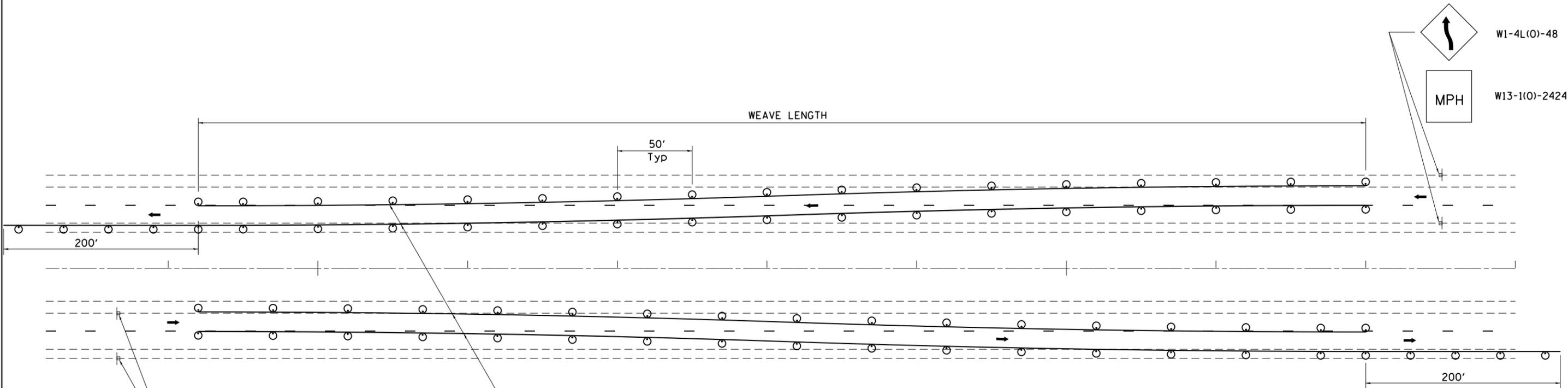
Temporary Pavement Marking required if Typical Weave is used for 14 days or more.
