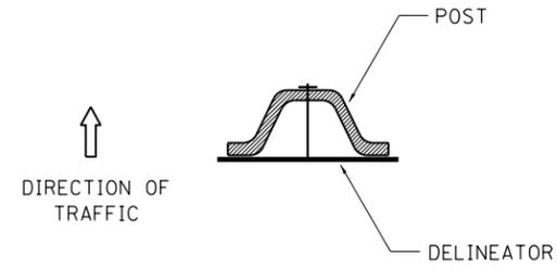
DELINEATORS SHALL BE INSTALLED ACCORDING TO STANDARD 635001 EXCEPT THAT THE POST SHALL BE ROTATED 180°. THE POST WILL HAVE THE WIDE SIDE FACING TRAFFIC AND THE DELINEATOR ATTACHED AS SHOWN ABOVE.
