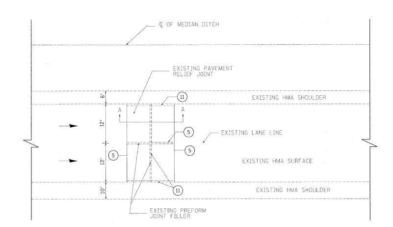
PLAN VIEW OF EXISTING PAVEMENT RELIEF JOINT
