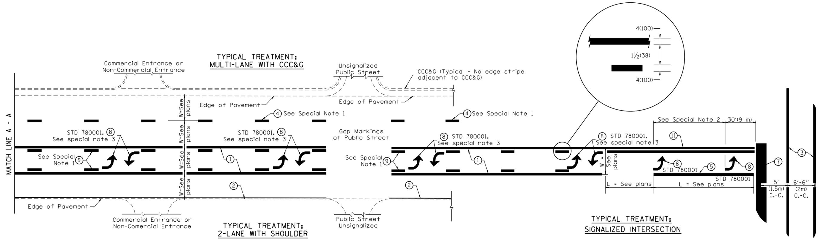
**FLUSH PAVED MEDIAN: TWO-WAY LEFT TURN LANE WITH ONE-WAY LEFT TURN LANE AT SIGNALIZED INTERSECTION**
