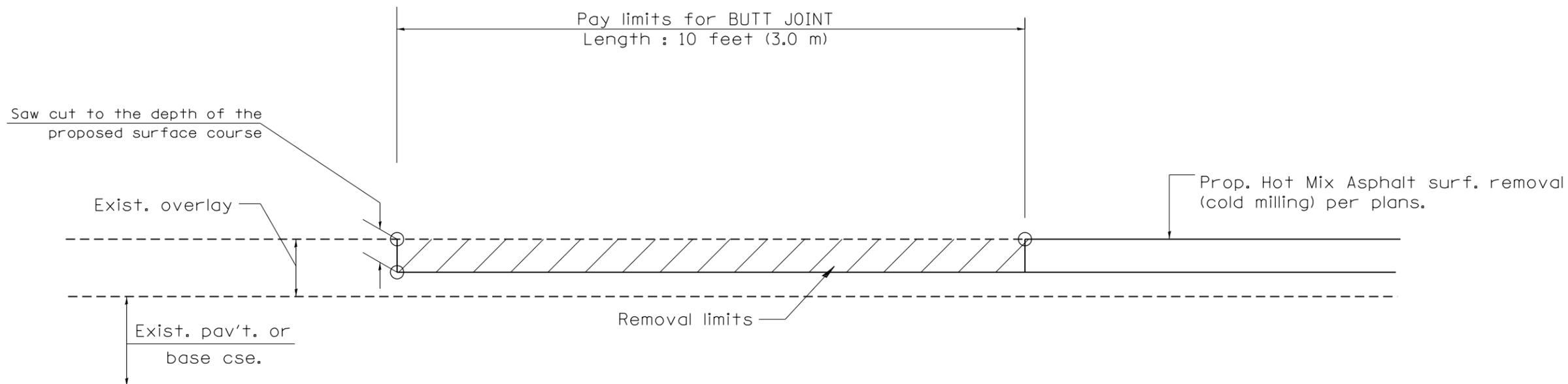
CASE 4 : SINGLE LIFT OVERLAY WITH EQUIVALENT DEPTH
